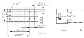
a) Indicated contact position during or after coil energization with reset voltage.
