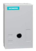
Non-reversing NEMA contactor, Size 00, Three phase full voltage, Contactor amp rating 9A, 3 wire (NO aux included), 110V 50Hz / 120V 60Hz coil, Non-combination type, Enclosure NEMA type 1, Indoor general purpose use, Standard width enclosure
