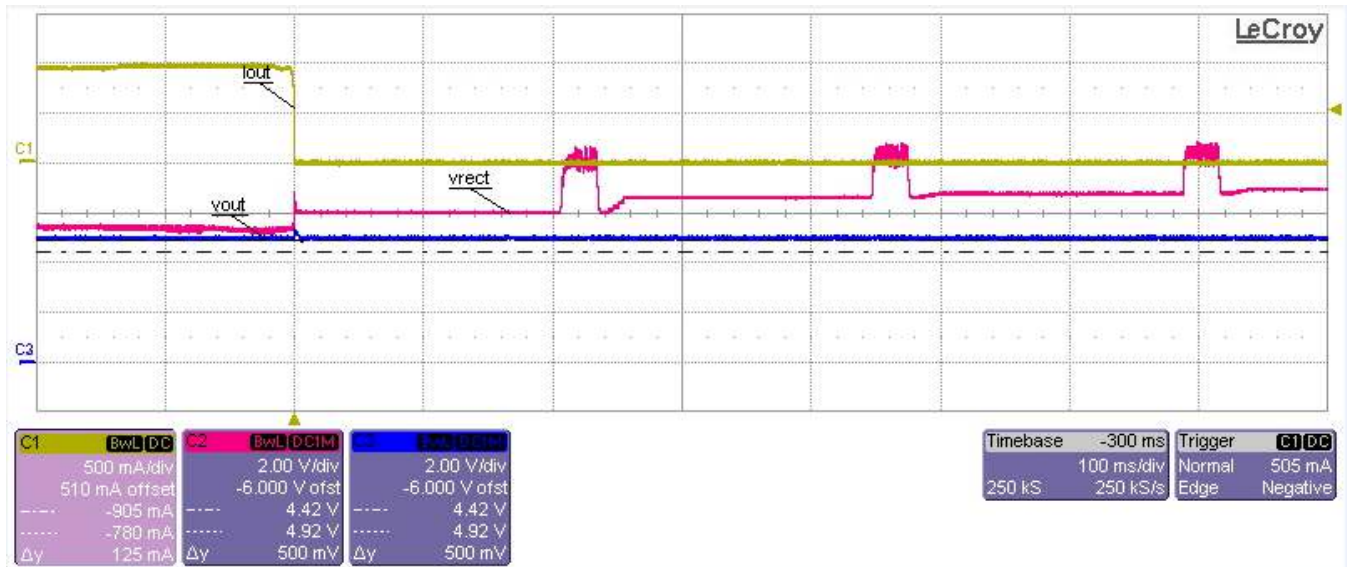
Figure 4. Load Dump, 500 mA to 0 mA
