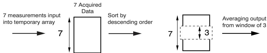
Figure 28. MAV Filter Operation (Patent Pending)
