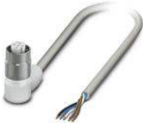
Sensor/Actuator cable, 5-position, PP-EPDM halogen-free, Gray RAL 7035, Free cable end, on Socket angled M12, A-coded, Cable length: 3 m, Hygienic design, With high-grade steel knurl
