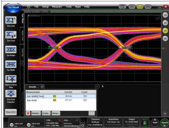
Figure 9. 5 Gbps Source Eye Diagram
