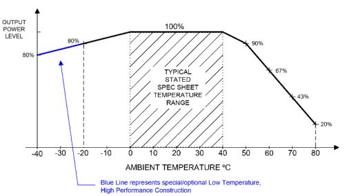
TYPICAL EXTERNAL POWER SUPPLY **DERATING CURVE** (GTM96900 LPS PRODUCTS)
