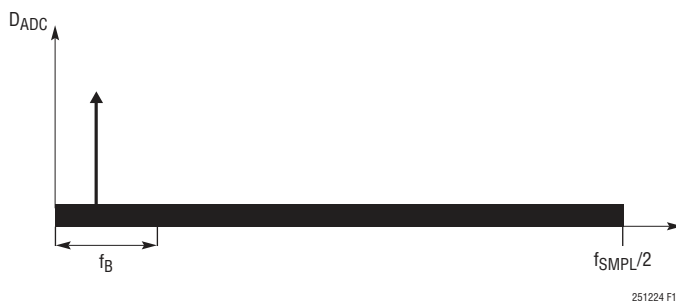
Figure 15. Frequency Spectrum of SAR ADC Core Output
