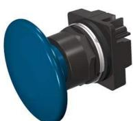
30mm BlackMax, Epoxy Coated Corrosion Resistant Metal Operator, Round Push-Pull Operator Non-Illuminated Mushroom Head Cap Large 2 1/2" (63.5 mm) Plastic, Blue 3 Position Pull-Momentary/Push-Maintained UL Listed, CSA Certified NEMA 1,3,3R,4,4X,12,13 & Automotive Standards
