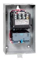
Non-reversing motor starter Size 1 Three phase full voltage Solid-state overload relay OLRelay amp range 5.5-22A 380-440/440-480V 50/60HZ coil Combination type Indoor general purpose use
