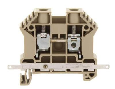
Feed-through terminal, Screw connection, Mounting type: Mounting rail TS 35/7.5, Rated cross-section: 16 mm², Width: 10 mm, Colour: Grey
