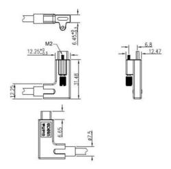
This cable includes a 10K pullup resistor between the 'CC' line and ' $V_{BUS}$ '. For systems compliant with the USB Type-C Cable and Connector Specification, the cable current will be restricted to 3.0A.
