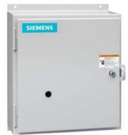
Non-reversing NEMA contactor, Size 2, Three phase full voltage, Contactor amp rating 45A, 3 wire (NO aux included), 220-240/440-480VAC 60Hz coil, Noncombination type, Enclosure NEMA type 12, Dust/drip proof for indoors, Extra-wide enclosure
