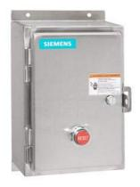
Non-reversing motor starter, Size 0, Single phase full voltage, Solid-state overload relay, OLRelay amp range 3-12a, 208VAC 60HZ coil, Non-combination type, Enclosure type 4X 304 S-steel, Water/dust tight noncorrosive, Standard width enclosure
