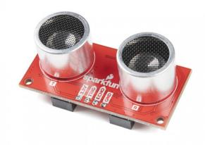
SparkFun Qwiic Ultrasonic Distance Sensor - HC-SR04
