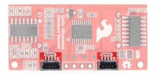
Ideally, power will be supplied via the Qwiic connectors on either side of the board. Alternatively, power can be supplied through the pins along the bottom side of the board labeled 3V3 and GND. The input voltage range should be between **1.8-3.6V**.
