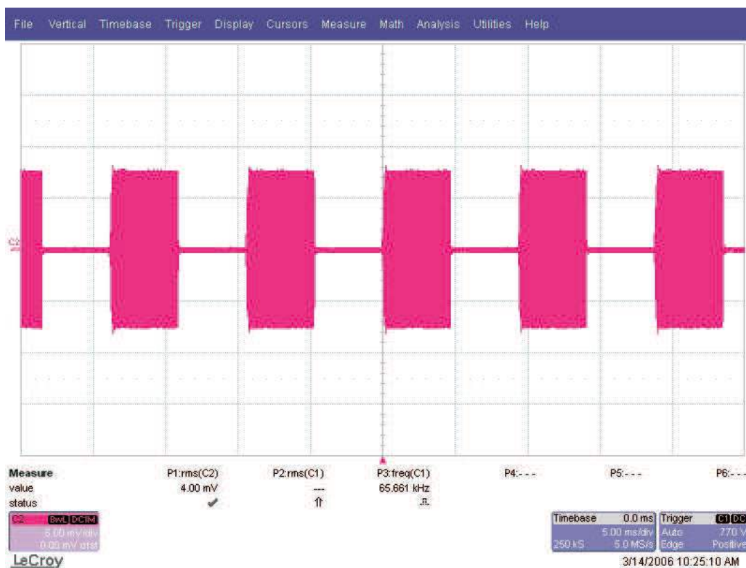
Figure 4. Burst Dimming Current at 50% Duty Cycle
