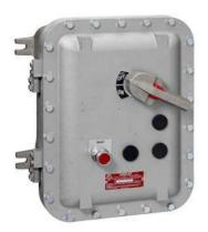
Non-reversing motor starter, Size 1, Three phase full voltage, Solid-state overload relay, OLR amp range 5.5-22A, 110V 50Hz / 120V 60Hz coil, Combination type, 30A fusible disconnect, 30A/600V fuse clip, Encl. NEMA type 4X fiberglass, Water/dust tight noncorrosive, Standard width enclosure
