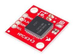
The breakout board allows for easy use of the HMC6343. All that is required is power (3.3V @ 4.5mA in run mode) and I2C connections to a microcontroller so that the module can receive commands and send data back to the user.
