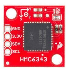
As you can see, the breakout has only four pins broken out. Two are for power, 3.3V and GND. Two are for I2C communication, SCL (clock) and SDA (data).
