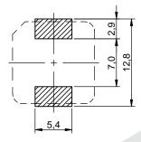
no sensitive traces underneath the component
