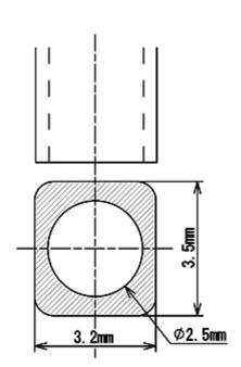
\*Nozzle with chamfering is recommended
