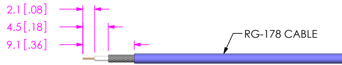
IN-PROCESS 1 STRIP CABLE AND TIN INNER CONDUCTOR
