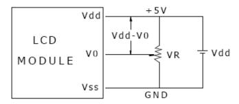
Vdd-V0: LCD Driving Voltage
