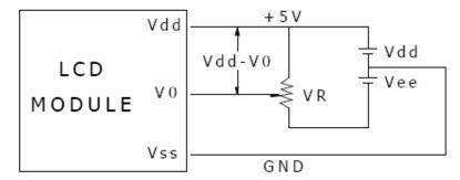
Vdd-V0: LCD Driving Voltage
