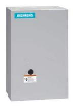
Electrically held lighting contactor, Contactor amp rating 30A, 0 N.C. / 6 N.O. Poles, 480VAC 60HZ coil, Non-combination type, (no disconnect device), Enclosure NEMA type 1, Indoor general purpose use
