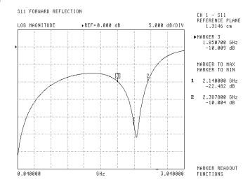
Figure 1. Standard Demo Board Return Loss
