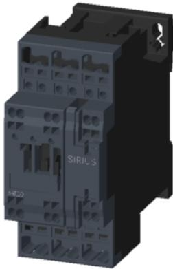
power contactor, AC-3 9 A, 4 kW / 400 V 1 NO + 1 NC, 110 V AC, 50 Hz 3-pole, Size S0 Spring-type terminal
