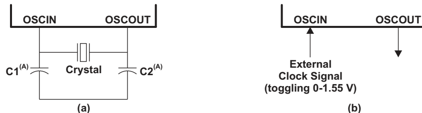
Figure 5-3. Recommended Crystal/Clock Connection
