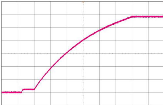
Figure 7. Rise time V_{SB} at 230VAC, full load (2ms/div) CH4: V_{SB} (2V/div)
