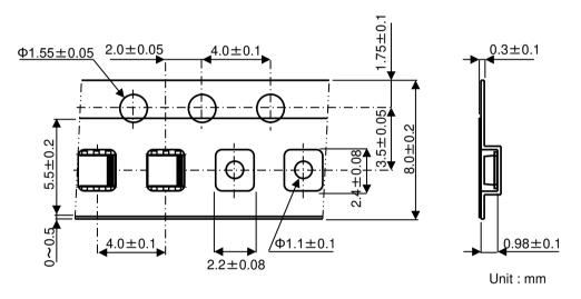
Note) Feed holes might be cover with the adhesive tape, but nothing will affect for using by that.
