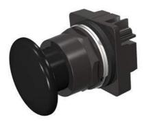
30mm BlackMax, Epoxy Coated Corrosion Resistant Metal Operator, Round Push-Pull Operator Non-Illuminated Mushroom Head Cap Small 1 3/4" (44.5 mm) Plastic, Black 3 Position Momentary UL Listed, CSA Certified NEMA 1,3,3R,4,4X,12,13 & Automotive Standards
