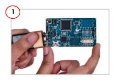
Connect the 9-V battery to the board.
