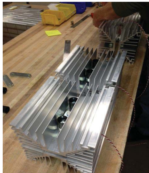
Fig. 8 - Step 6: Check to make sure the two mounting surfaces are still parallel. Tighten each bolt a 1/10 th turn more. Do not tighten beyond this point.
