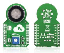
Air quality click<sup>™</sup> is a simple solution for adding a high sensitivity sensor for detecting a variety of gases that impact air quality in homes and offices. The board features an MQ-135 sensor, a calibration potentiometer, a mikroBUS<sup>™</sup> host socket, two jumpers and a power indicator LED. Air quality click<sup>™</sup> communicates with the target board through mikroBUS<sup>™</sup> AN (OUT) line. Air quality click<sup>™</sup> is designed to use a 5V power supply only.
