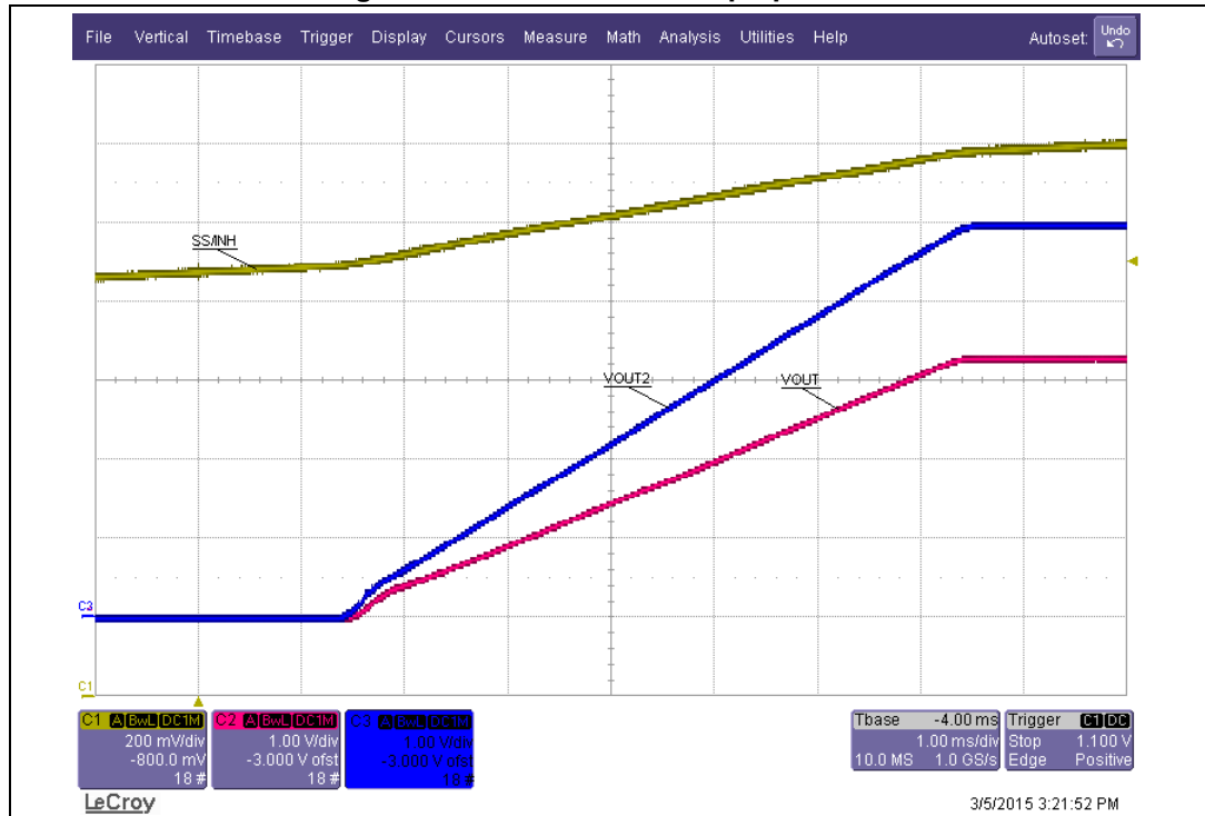
Figure 11. Ratiometric startup operation
