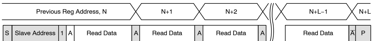
Figure 38. Single READ from Current Location
