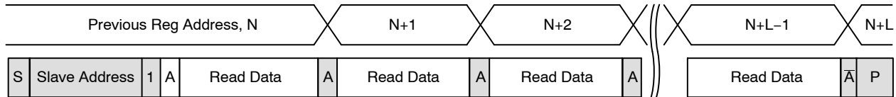
Figure 40. Sequential READ, Start from Current Location
