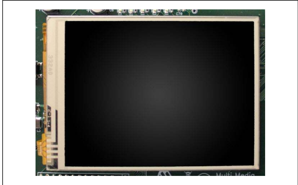
FIGURE 2-3: 3.2 INCH (8.1 CM) QVGA TFT TOUCH SCREEN
