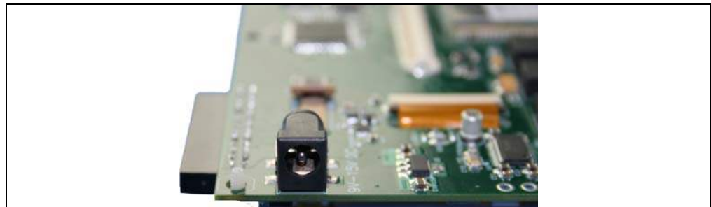
FIGURE 2-1: DC POWER SUPPLY
