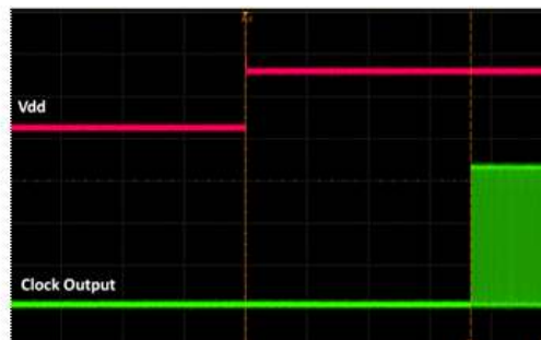
Figure 16. Startup Waveform vs. Vdd
