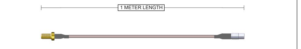
Connector A 132117 SMA Jack Straight Brass Gold + Heatshrink 50 Ohm RG-316 Continuity/Hi-Pot Connector B 252138 MCX Jack Straight Brass Nickel + Heatshrink
