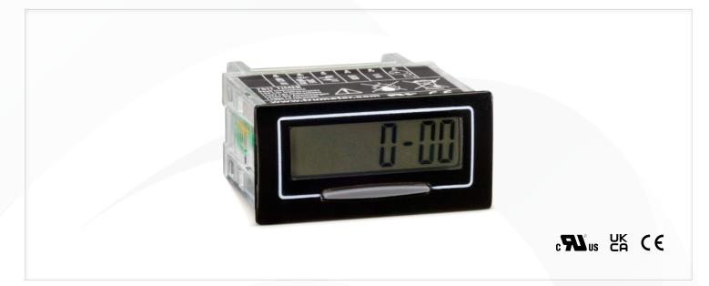
8-digit liquid crystal display timer, self-powered with a 10-year battery life. A compact LCD timer designed for many applications, screw terminals ensure fast wiring. Features include backlighting (external 5VDC supply required), 4 timing modes, timing direction indication and 9mm high digits. High Voltage (HV) version accepts input voltages of 5-110VDC or 10-240VAC.
