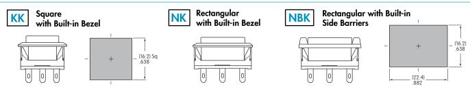
Snap-in Mounting with Solder Lug terminals is the standard combination. Panel Thickness: 1.0 ~ 3.2mm (.039 ~ .126")
