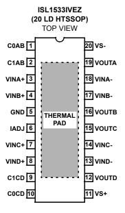
THERMAL PAD TO BE CONNECTED TO GND
