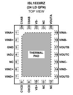
THERMAL PAD TO BE CONNECTED TO GND
