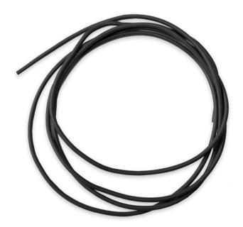
• Mueller's WI-M-20-@ is 20 AWG, 41/0.127 stranded, tinned copper wire with highly flexible 0.088" (2.24mm) diameter silicone jacket.
