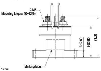
Main contact terminal connection and coil connection with positive and negative difference.
