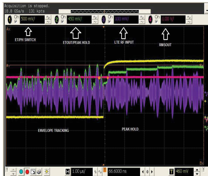
Figure 19. RMSOUT, Envelope Tracking, Peak Hold Performance with LTE signal @ 1900 MHz
