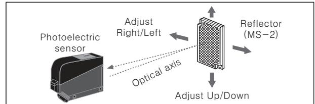
※ If use more than 2 photoelectric sensors in parallel, the space between them should be more than 30cm.
