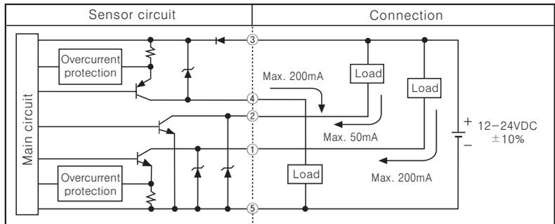
※In case of product with the output protection device, if terminals of control output are short-circuited or overcurrent condition is existed, the control output will turn off due to protection circuit.
