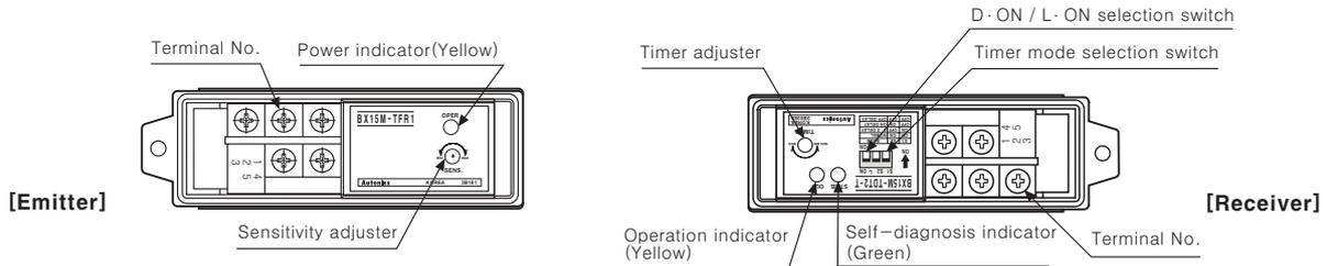
○Retroreflective / Retroreflective with polarizing filter ○Diffuse reflective
