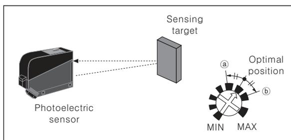
※ The sensing distance indicated on specification chart is against  $200 \times 200\text{mm}$  of non-glossy white paper. Be sure that it can be different by size, surface and gloss of target.
