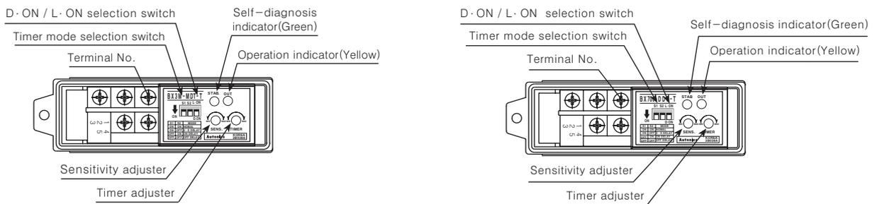
※There are no Timer mode selection switch and Timer adjuster in type without Timer function.
