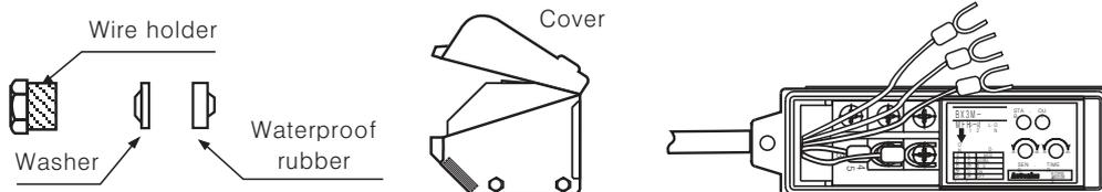
※ On servicing wire, connect wire on terminal as above figure.
