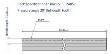
There is no provision for option racks complying with the gear specification G2 (shifted spur gear) of FRN-P2
