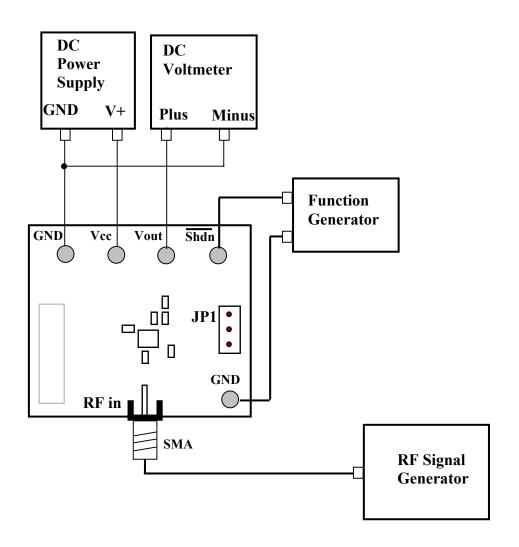
DC539A Demo Board Connection Diagram
