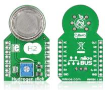
Hydrogen click<sup>™</sup> is a simple solution for adding a high sensitivity hydrogen (H<sub>2</sub>) sensor to your design. It's suitable for designing gas leakage equipment. The board features an **MQ-8** sensor, a calibration potentiometer, a **mikroBUS<sup>™</sup>** socket and a power indicator LED. Hydrogen click<sup>™</sup> communicates with the target board through mikroBUS<sup>™</sup> AN (OUT) line. Hydrogen click<sup>™</sup> is designed to use a 5V power supply only.
