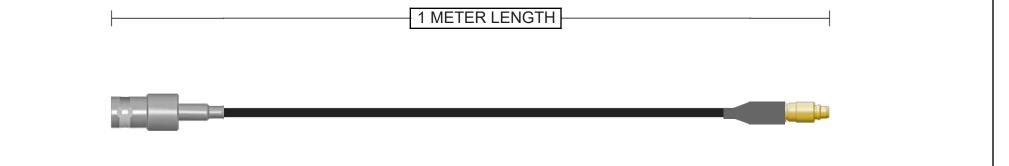
Connector A 112160 BNC Jack Straight Brass Nickel 50 Ohm RG-174 Continuity/Hi-Pot Connector B 262101 MMCX Plug Straight Brass Gold + Heatshrink
