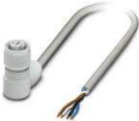
Sensor/Actuator cable, 4-position, PP-EPDM halogen-free, Gray RAL 7035, Free cable end, on Socket angled M12, A-coded, with 3 LEDs, Cable length: 1.5 m, Hygienic design, with plastic knurl
