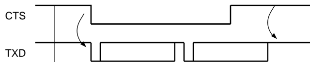
Figure 34-29. Transmitter Behavior when Operating with Hardware Handshaking
